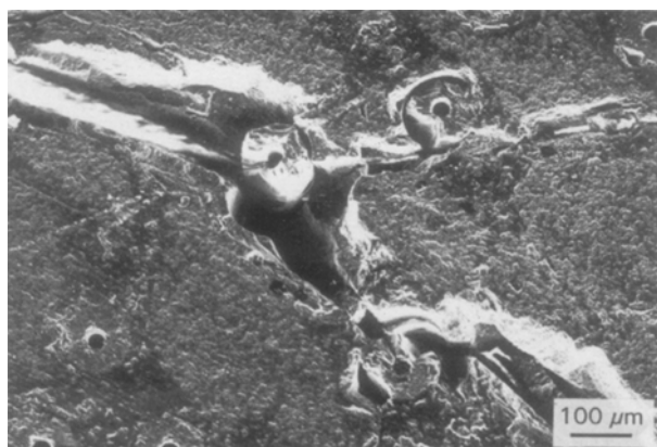
Figure 7 SEM micrograph of the crept SiC fibre/AlN composite. Note that crack was initiated at the reacted region of the SiC fibre and matrix.
